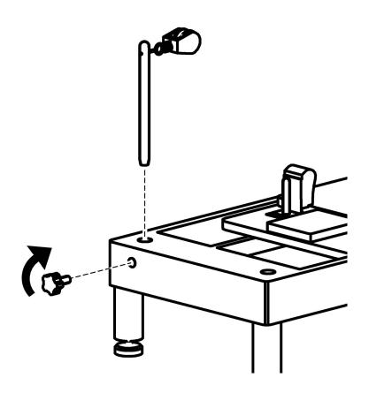
Keeping at least one carriage spring attached for safety; next add the shoulder rests and secure them using the shoulder rest securing poles.
