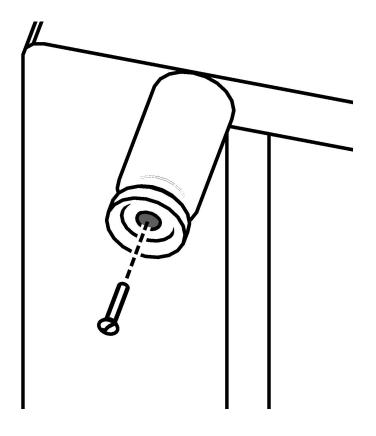
Then tighten the barrel of each leg with your hand.
