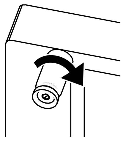
You can now safely adjust the height of your reformer by turning the foot.
