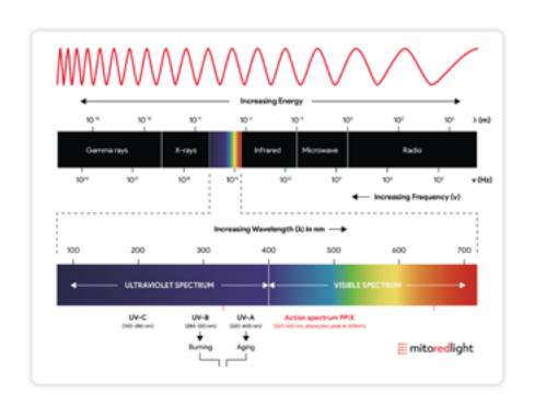
If you remember high school physics, when you pass white light through a prism it separates out the different colors based on their wavelengths (ROYGBIV). Only a tiny part of this spectrum (roughly 400nm to 700nm) is actually visible to the human eye.
