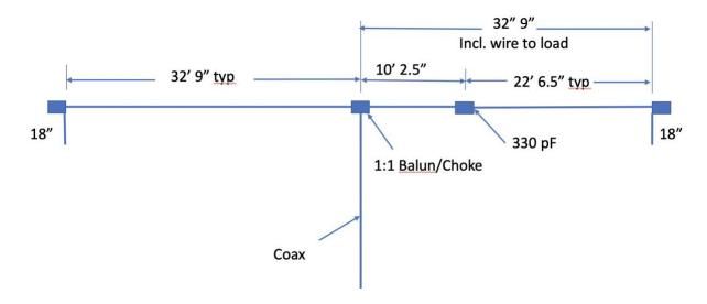
Modified Existing 40M Dipole to 40M & 15M Dipole
