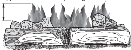
Figure 31 - Correct Burner Flame Pattern
