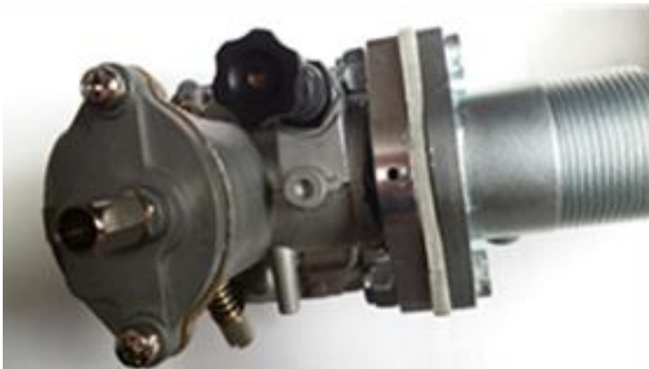
Top picture showing heat insulator and lock nuts on Triumph manifold.
