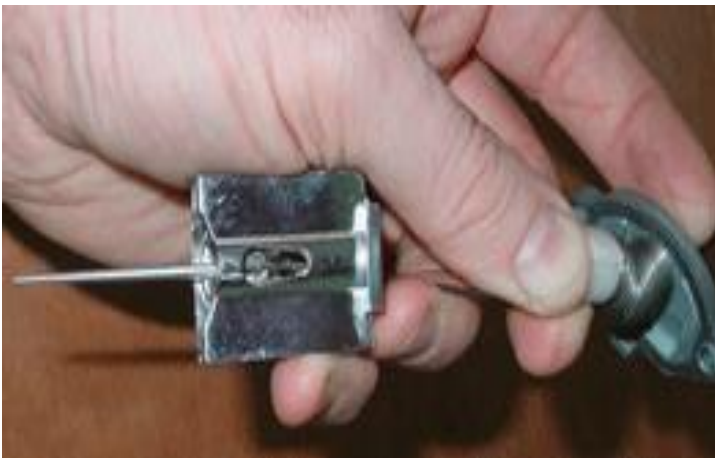
Fig. 4 Now insert the end of the cable so that the nipple sits in its place in the throttle slide.
