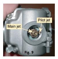
To replace the main jet, the bottom large nut at the base of the float bowl can be removed, Fig.9 (remember to turn off your fuel tap from the tank). Some fuel will spill out so have a large rag or bowl to catch it. A couple of small spanners will be needed to remove the jet.
