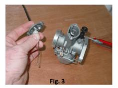
Having removed the top cover, push the nipple end of the throttle cable through the top cover and down the center of the spring and through the white retaining collar. Note that the white retaining collar must be installed the same direction it comes out. Compress the spring and hold it all together so as much of the cable is showing as possible.
