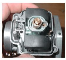
For changing of the pilot jet, the float bowl needs to be removed to gain access to it and this can be done by removal of the two screws. NOTE – the bowl needs to be gently maneuvered around to release it as there are the floats and internal structure inside. This must be done very gently for both removal and reinstallation. Fig. 10 shows what is there once the bowl is removed (in the photo the carburetor is removed from the bike and sitting on a bench).
