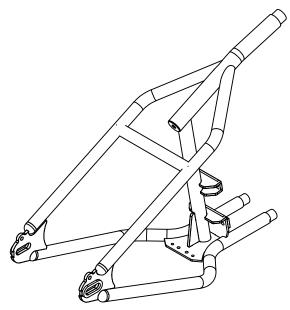
Installation of this hardtail frame is easy and takes only an afternoon. All tubing matches the stock frame tubing diameter, with a 1-5/8 inch thick walled steel backbone and 1-1/4 inch diameter heavy-duty lower frame rails. This blends the installed hardtail seamlessly into your stock frame.
