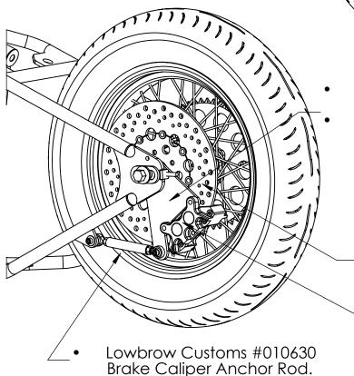
Lowbrow Customs #010583 Rear Caliper Bracket for 11.5" Rotor Black. Lowbrow Customs #010584 Rear Caliper Bracket for 11.5" Rotor Raw.
