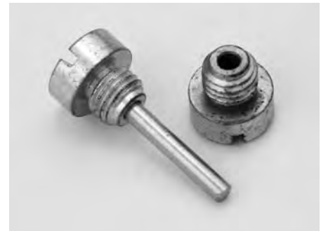
Carburetor Float Lever Screw Kit Cadmium plated screw with rod, OEM 27383-11 and screw, 27384-16, used on 1916-1965 Schebler and Linkert carburetors. Stock No. 2827-3
