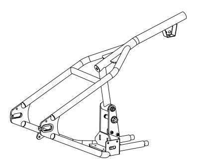
The Gasbox hardtail frame conversion kit is engineered using the latest CAD technology for high strength, a perfect fit and easy installation. The backbone is thick walled 1-5/8" steel, lower tubes are CNC bent thick walled 1-1/4". The seat post is 1-1/2" diameter. The unique rear engine mount eliminates the stock rubber mounts and cleans up the design for a lean chopper look. All plates are precision CNC laser cut and TIG welded.
