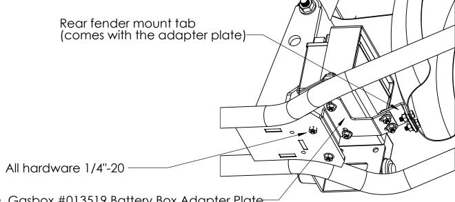
Gasbox #013519 Battery Box Adapter Plate.
