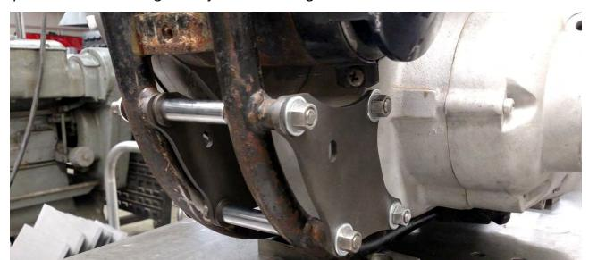
5. Check your tube alignment and adjust for the best fit. The gas tank hole centers should match your measurements of 16-5/8".
