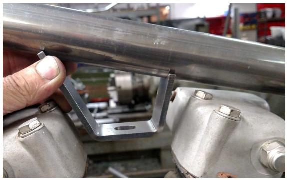
8. Locate and weld the disc brake tab for a custom fit.
