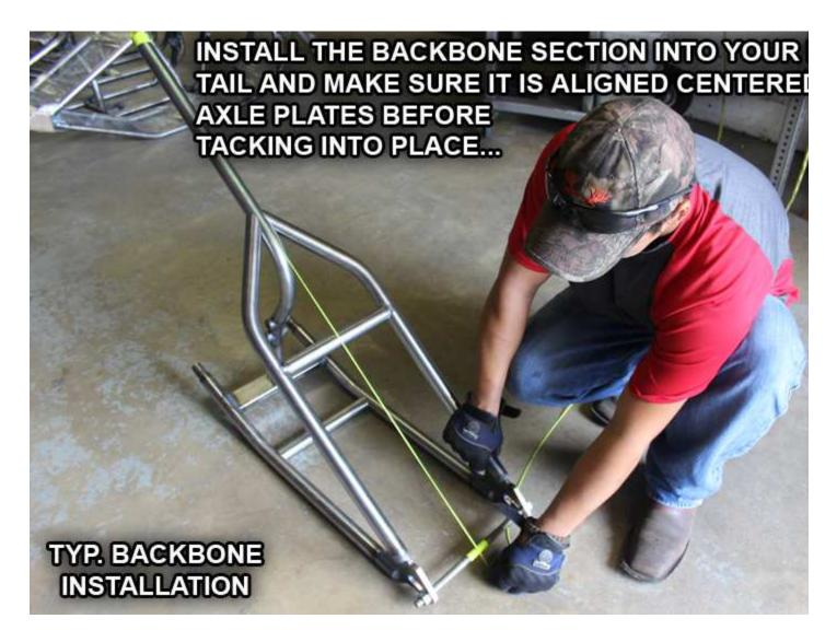
Once your backbone is tacked in place, the hardtail section should resemble this... Be sure NOT to fully weld the seat post connections (top or bottom) until the hardtail is fitted to the frame.
