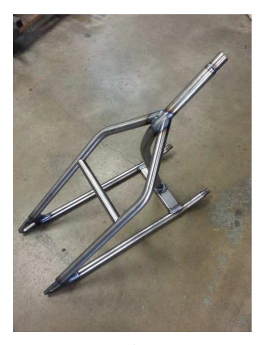
When installing the hardtail to the frame, make sure the complete assembly is IN LINE with the original frame
