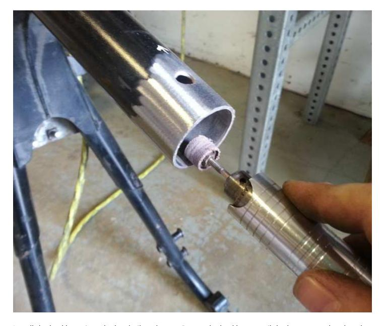
Install the backbone into the hardtail as shown. Rotate the backbone until the bottom can be placed inside the cut hole on the cross member.
