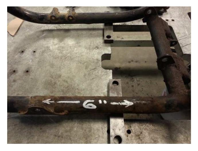
Next, you will clean the INSIDE and OUTSIDE of all three cut locations and drill your plug holes for welding the hardtail in place.
