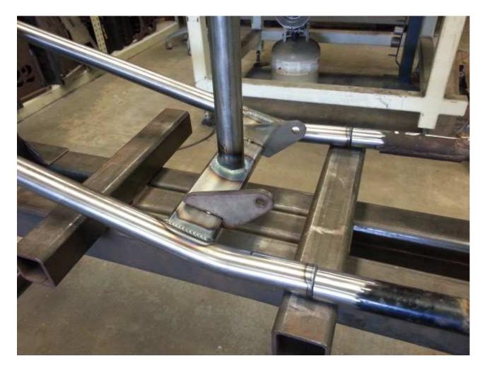
Once your rear motor mounts have been tacked in place, remove the motor for the final time and fully weld everything.
