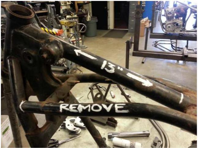
Then, from the centerline of the motor mount, measure 6" toward the rear of the frame and scribe. The frame will then be cut top and bottom on all three marks.
