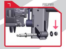
Torque to 40 ft. lbs. Using 18mm. 6mm hex wrench will prevent bolt rotation.
