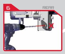
Drill outside tab only using a 5/8" drill bit.
