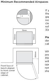
If you have a cupboard above the refrigerator with a rear gap of less than 100mm (Y), recommended minimum clearance at the top of the refrigerator increases from 30mm to 70mm (X).
