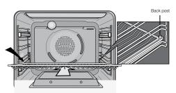
2. Drop the front of the shelf or tray onto the slide ensuring it sits behind the front post of the slide.
