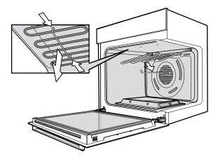
NOTE: Diagram shows a grill in oven model. Separate grill models use the same hanger clip arrangement in the grill compartment.
