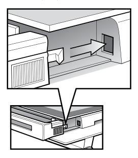
3. Push the middle of the trim down to ensure it is straight and firm against the glass panel.
