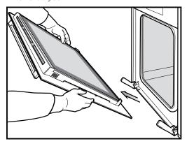
4. Lay the oven door with the outer side facing downwards on something soft and flat (for example a blanket on a kitchen table) to prevent scratches.
