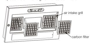
Optional carbon filters diminish cooking odours in the recirculated air. Depending on the frequency of use and the type of cooking, the expected life of carbon filters is 3 months. Using carbon filters will reduce the airflow of the angehood.
