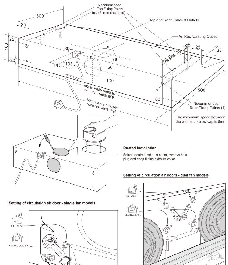
IMPORTANT: SET CIRCULATING MODES BEFORE INSTALLING THE HOLE PLUGS.
