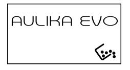
If the drawer is not emptied after several brewing cycles, the machine will stop and the display will show:
