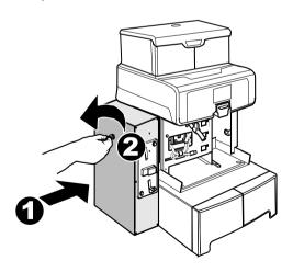
Insert the front cover and fix it by means of the screw previously removed. Insert the coffee dispensing spout. Reassemble the drip tray.
