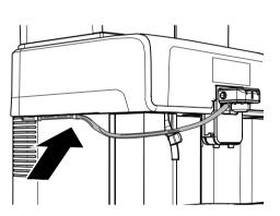
If the coiner is installed, fix the tube as shown in the figure by using the previously removed cover.
