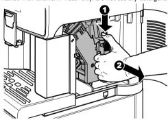
Wash the brew group with lukewarm water; carefully wash the upper filter. Before placing the brew group in its seat, ensure that there is no water left in the brewing chamber.
