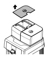
Remove the tank; lift it using the inside handles.
