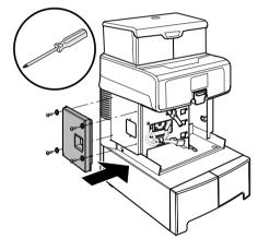
The machine has two different connectors, a square-shaped one for the "Apollo" payment system and a rectangular one to connect the coiner.
