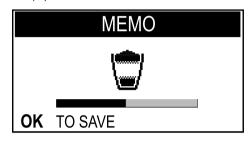
Press the "OK" button when the desired amount of milk is reached in the cup.
