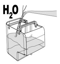
When filling the water tank, use sterile disposable gloves to prevent bacteriological contamination.
