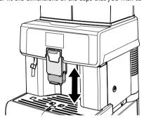
Manually move the dispensing spout up or down to adjust its height.
