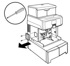
Install the spacer on the left-hand side of the machine and fix it using the 4 screws supplied.
