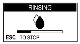
Wait for this cycle to be completed automatically. The dispensing process can be stopped by pressing the "ESC" button.
