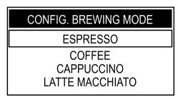
Select the beverage that you wish to program and stop the brewing process when desired, as shown on the display.
