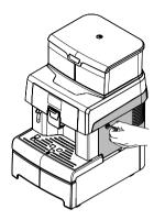
Remove the brew group by pulling it by the handle and pressing the «PRESS» button. The brew group must be washed with lukewarm water only. Do not use any detergent.
