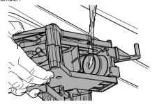
Lift the rear side of the inner drawer to unlock it.
