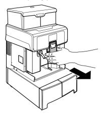
Remove the front cover by pushing on its sides to disengage the fixing elements.
