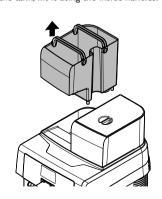
Rinse and fill it with fresh water; do not exceed the level (MAX) indicated on the tank.
