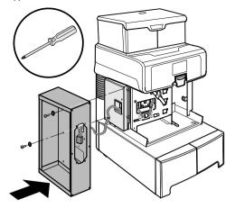
The connecting cable must be properly inserted in the box.
