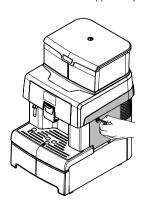
Remove the brew group by pulling it by the handle and pressing the «PRESS» button.
