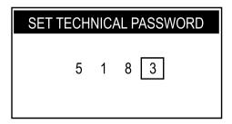
When the "OK" button is pressed on the last number, the machine saves the code and displays the following page.
