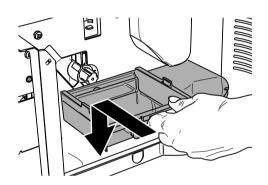
When fitting the drawer, carry out the same operations performed for its removal, but in reverse order.
