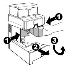
Remove the lid on the left-hand side by loosening the 2 screws.
