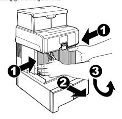
Install the sensor on the inner side of the front cover. When the sensor has been installed, connect it.
