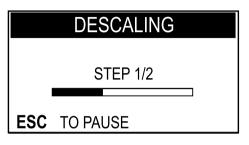
If you do not have a container of this capacity, pause the cycle by pressing the "ESC" button, empty the container, put it back onto the machine and restart the cycle by pressing the "OK" button.
