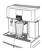
Before brewing any product and/or when bringing the dispensing spout back to its normal position, ensure that it is correctly positioned. This can be evidenced by the CLICK indicating correct positioning.
