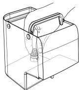
Put the filter into the empty tank. Press it to its limit stop.
