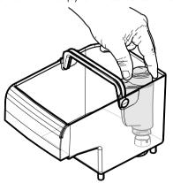
Fill the tank with fresh drinking water and reinsert it into the machine.
