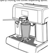
When the machine is ready, press the "Milk" button to start dispensing the hot milk.
