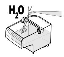
When filling the water tank, use sterile disposable gloves to prevent bacteriological contamination.
