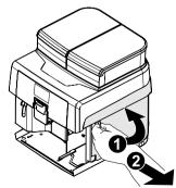
Remove the brew group by pulling it by the handle and pressing the «PRESS» button.
