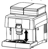
Manually move the dispensing spout up or down to adjust its height.
