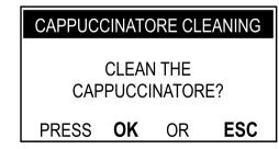
Press the "OK" button to start the Cappuccinatore cleaning cycle. Follow the instructions on the display.
