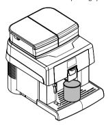
Press the "Coffee" button to start brewing. The machine starts brewing coffee from the dispensing spout. Wait until brewing has been completed and empty the container. Repeat the brewing process 3 times.
