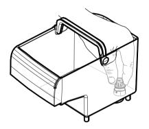
Put the filter into the empty tank. Press it to its limit stop.
