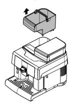
Rinse and fill it with fresh water; do not exceed the level (MAX) indicated on the tank.
