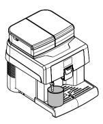
Press the "Hot Water" button to start dispensing HOT WATER.
