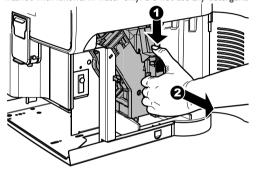
Wash the brew group with lukewarm water; carefully wash the upper filter. Before placing the brew group in its seat, ensure that there is no water left in the brewing chamber.
