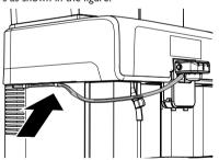
Clean the suction hose externally with a damp cloth. This way, all parts will be perfectly clean and free of any milk residue.
