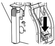
Make sure that the hook which locks the brew group is in the correct position. firmly press the "PRESS" button to check its position.
