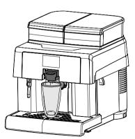
Before brewing any product and/or when bringing the dispensing spout back to its normal position, ensure that it is correctly positioned. This can be evidenced by the CLICK indicating correct positioning.
