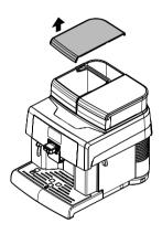
Remove the tank; lift it using the inside handle.
