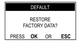
The restoring operation permanently deletes the stored data. To exit the procedure, press the "ESC" button.
