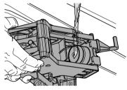
Lift the rear side of the inner drawer to unlock it.
