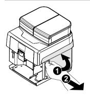
Remove the brew group by pulling it by the handle and pressing the «PRESS» button. The brew group must be washed with lukewarm water only. Do not use any detergent.
