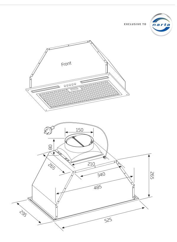
Model:NAUM-6, NAUM-6BFeeding Voltage:220-240V 50HzMax Lamp Power:2 x 1.5W
