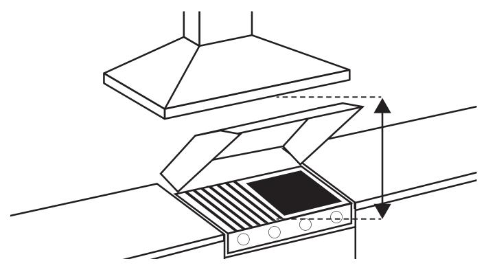
Measurements are from the top of the trivets to the lowest part of the rangehood, including the button controls.
