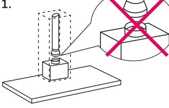
Never reduce flue diameter right next to the rangehood outlet fitting.
