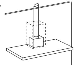
Straight ducting is the most effective installation
