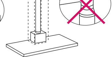
Never fit reductions next to curves or bends in the installations. They must always be in straight sections and as far as possible from the rangehood.
