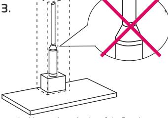
Avoid excessive reduction of the flue size, as this drastically reduces extraction capacity.
