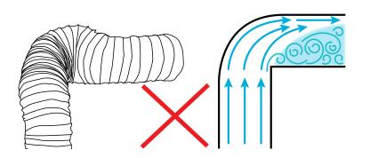
Crushed or kinked ducting creates sharp corners that creates turbulence. This reduces the size and efficiency of the ducting, lowers extraction and may cause excessive noise.
