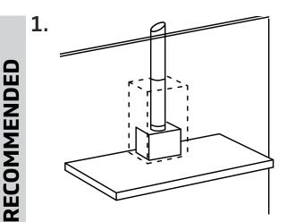
Straight ducting is the most effective installation
