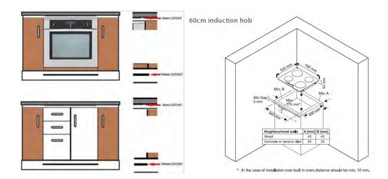
If there is access to the cooktop base (for example, through a cupboard), a board must be placed a minimum of 30mm below the cooktop that prevents anyone from touching the cooktop base. The board must comply with the ventilation requirements above, and be removable, to allow access during maintenance etc
