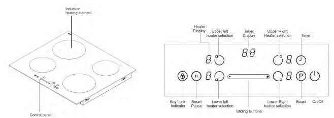
The induction cooktop appliance is operated by touching buttons, with the functions confirmed by LED displays and acoustic signals.
