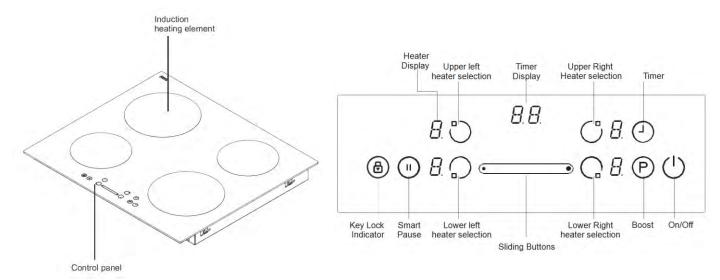
The induction cooktop appliance is operated by touching buttons, with the functions confirmed by LED displays and acoustic signals.
