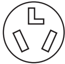
3-wire receptacle (10-30R)
