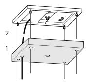
Slowly loosen **adjusting screws** and align rangehood horizontally. Tighten the wire ropes evenly.
