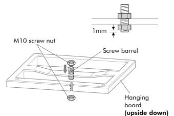
**3** Attach 4 adjustable screws to the hanging board. Align the screw and do not over tighten.
