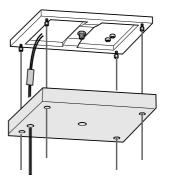
Secure connected wires with insulating tape.
