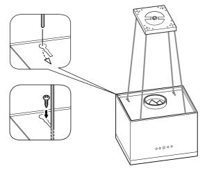
9 Loosen the cover lock nut
