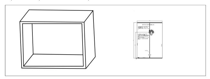
2. Make the marks on the bottom plane of cabinet according to marks "a" on the template
