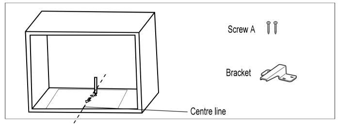
3. Remove the bottom cabinet template and fix the bracket with screws A.
