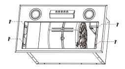
Unfastening the screws (ST4\*10), remove the lid of terminal box, disconnect the wires to the Commands at the connectors.
