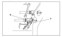
Clean the cone and it's slot by means of a cloth soaked with solvent. Slightly grease the cone with the relevant grease, put it in it's slot, and turn it a few times. Remove the cone again, remove the excess grease making sure the gas entries are not obstructed by grease residue. Assemble everything carefully in the opposite direction check the connection seal by means of soapy water.
