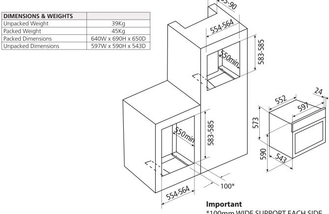
\*100mm WIDE SUPPORT EACH SIDE WITH 50mm CLEARANCE UNDERNEATH
