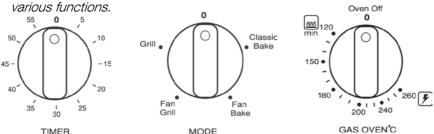
'TIMER': Minute counter – rotate the knob to the desired time up to 60 minutes and a bell will ring at the end of the time period. For very short time periods turn the knob past the point you want and then back to it to load the timer mechanism. Some models may have an electronic timer. Refer to electronic timer instructions in this book.
