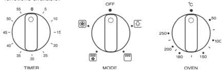
TIMER: Minute counter – rotate the knob to the desired time up to 60 minutes and a bell will ring at the end of the time period. For very short time periods turn the knob past the point you want and then back to it to load the timer mechanism. Some models may have an electronic timer. Refer to electronic timer instructions in this book.
