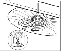
**CAUTION!** An incorrect position of the filters can cause bad washing results and damage to the appliance.
