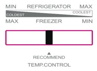
All cold air is coming from freezer compartment, there is an air flow adjustment knob on the back panel.
