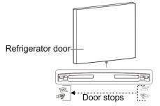
11. Install the refrigerator compartment door.
