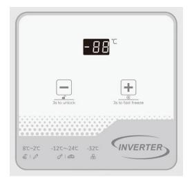
When the system is powered on for the first time, all LED indicators and the digital display light up, and will restore to normal display in 2s. When the digital display screen is on, it will automatically go off if no key operation within 3 minutes, with all keys locked. When the display screen is off, you can wake it up by pressing any key. **Hold down the "-" key for 3 seconds to unlock the keys**.
