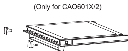
Removal of the internal glass panel
