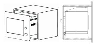
Open the door of the microwave oven. Use the provided screw to fasten the microwave oven to the cabinet and place the plastic
