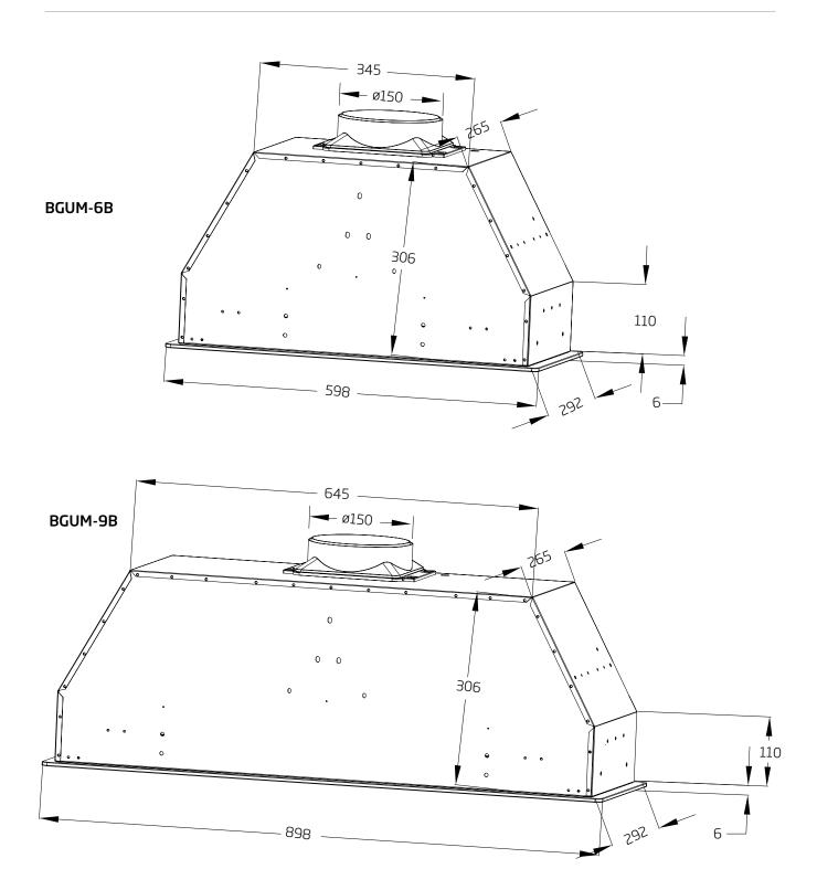
Model: BGUM-6B, BGUM-9B Feeding Voltage: 220-240V 50Hz
