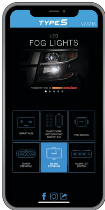
Tap “SMART EXTERIOR” icon to start. The APP will automatically pair to the Smart Hub when the Wheel Well Lights and your device are powered on and within the 30-foot Bluetooth® range. We strongly recommend that you setup a private password to prevent unauthorized devices from connecting to the Smart Hub. (Refer to password instructions on page 17)
