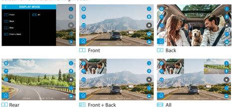
**NOTE:** "Rear" mode and "All" mode only available when the add-on 1080P Rear Cam (BT532838) is connected.
