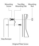
Warning: Lower tailgate on pickup trucks slowly and check for minimum ¼ inch clearance between gate and top of camera frame. This check is because some bumpers are installed higher than others.
