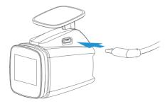
6 Route the power cable to your 12/24V outlet (cigarette lighter) and hide the cable in the headliner and pillars. We recommend going through the passenger side so the cable doesn't get into the driver's way.
