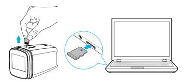
Please power off the Dashcam and detach it from the Magnetic Mount. Remove the MicroSD card and connect it to your computer via a MicroSD card adapter or reader (not included). Once connected, the MicroSD card will appear as a removable storage device.
