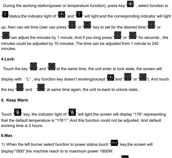
2) When the left burner select function to temperature status, touch " $^{Max}$ " key, the screen will display "464", the machine reach to maximum temperature 464°F.
