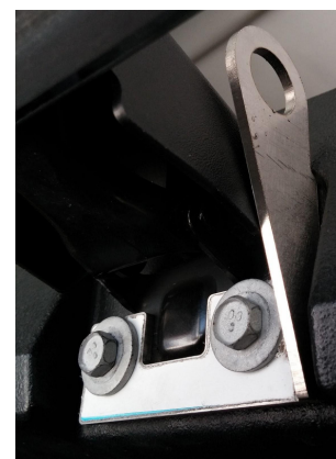
(Hinge Bracket shown un-painted for contrast)
