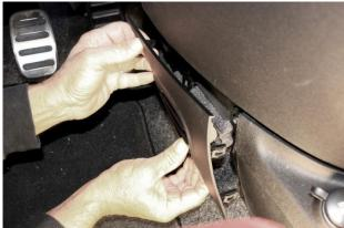
Remove the T25 Torx screw from driver side lower cover then pull off.
