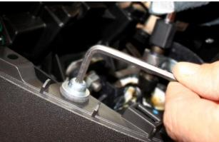
Remove the T25 Torx screw and 5mm Hex Key bolt from each side on the top edge of console.
