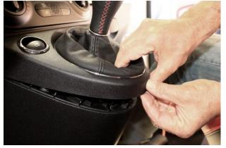
1. Grab the rear of the center console top and lift up to detach.
