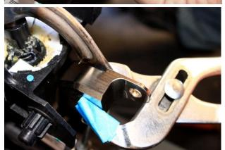
Install neu-f billet adapter onto lever, should be a snug fit.
