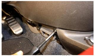
With cover removed, remove exposed T25 Torx screw.
