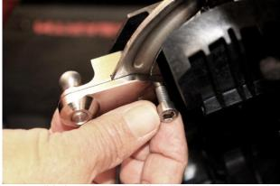
Install locking plate with cable ball end and M6x16 Socket Cap screw. Tighten evenly using 9/16" open end wrench and 5mm Hex Key wrench.
