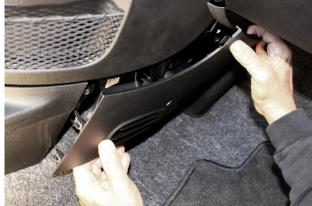
Remove the T25 Torx from passenger side lower cover then
