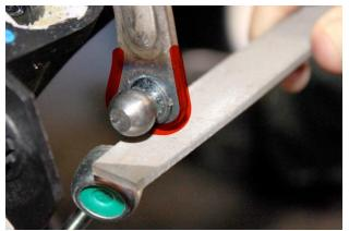
9. Using a metal file, go around the outside edge of the shift lever stamping to remove any burrs or high spots.
