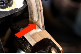
11. When adapter is fully seated on lever there should be no gap at the top edge.
