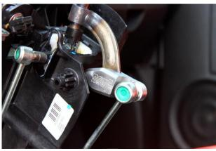
13. Grease ball and push on cable socket end. Check operation of shifting thru gears.
