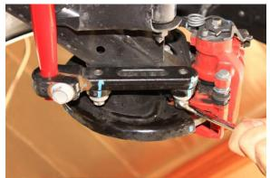
Insert neuf torsion bar into driver side mount then reinstall passenger side mount. Center torsion bar and torque mounting bolts to 108Nm (80 Ft. Lbs.)
