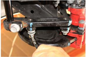
Using E18 Torx wrench unbolt passenger side torsion mounting bracket. Then pull out bar from driver side mount. NOTE: Not the correct tool but a 14mm box end wrench is possible to use.
