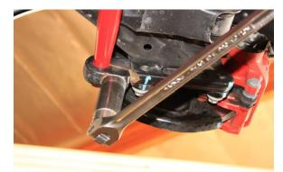
6. Tighten and torque both 21mm Hex bolts to 190Nm (140 Ft Lbs.)
