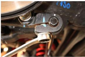
3. Generously loosen the 21mm Hex bolt on each end of the original torsion bar.
