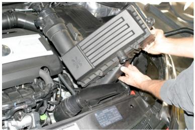
1. Remove air filter box to access factory shifter lever.
