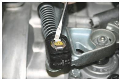
2. Remove clip by prying up the center tab with small flat head screw driver and sliding the clip sideway.
