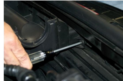
8. Lift off lower air filter box from rubber grommet mounts, then lift out left side first and rotate intake duct around small coolant hose to remove.
