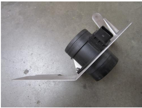
13. Mount MAF sensor to SS P-Flo bracket using supplied M6x16mm screws and lock nuts, then tighten.
