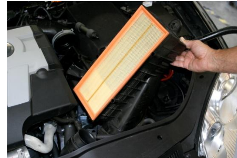
8. Lift off lower air filter box from rubber grommet mounts, then lift out left side first and rotate intake duct around small coolant hose to remove.
