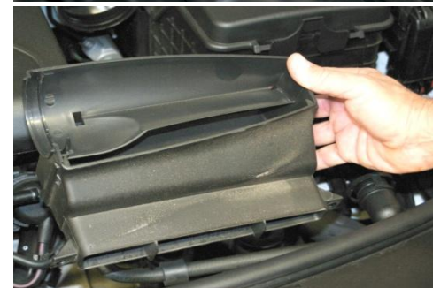
9. Remove air intake duct at radiator support (2) T25 Torx, one on each side.
