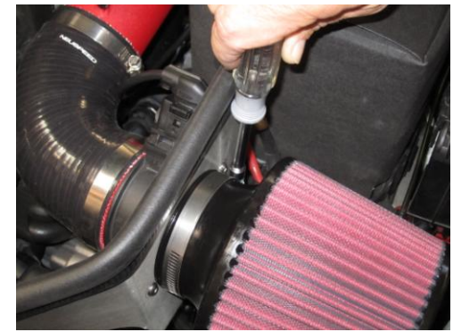
23. Attach and tighten NEUSPEED filter. Position NEUSPEED logo on end of filter horizontally.
