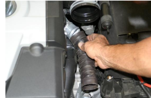
10. Remove hot air ducting hose.
