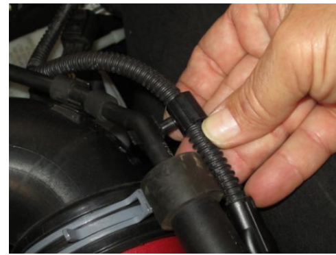
20. Move MAF wire harness support clip down next to vacuum canister.
