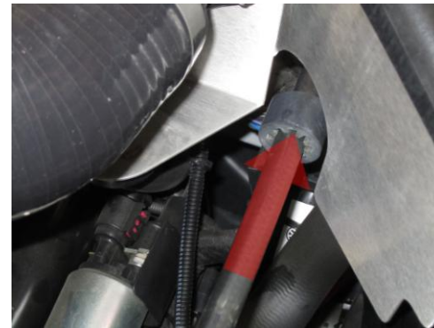
22. For extra protection, slide coolant hose protector sleeve just under P-Flo bracket.
