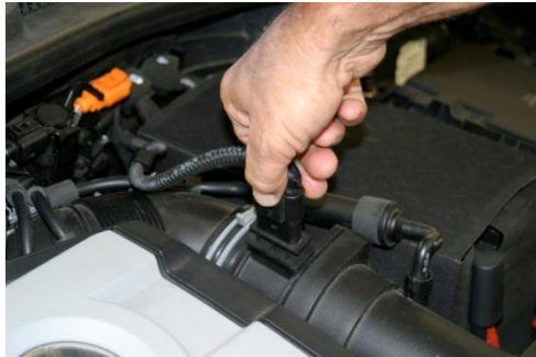
1. Disconnect Mass Air Flow (MAF) sensor electrical connector.
