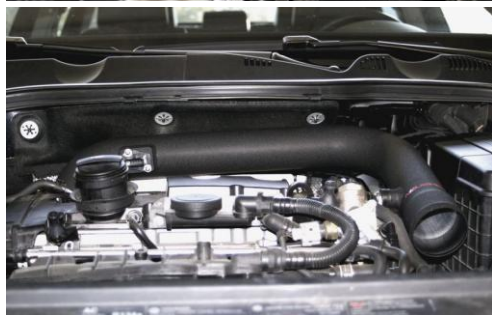
14. Slide coolant hose down in retaining clamp just before molded bend in hose.
