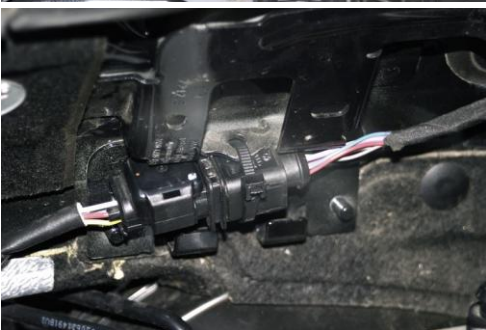
11. Remove O 2 sensor connector from clip at firewall. Pull off plastic harness clip from firewall. Wire-tie O 2 sensor harness to firewall bracket as shown.
