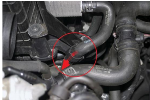
14. Slide coolant hose down in retaining clamp just before molded bend in hose.
