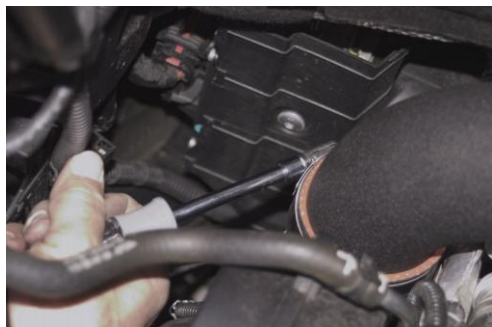
12. Install NEUSPEED intake pipe onto turbo inlet with #44 clamp supplied and attach rubber isolator mount to ear on end of cylinder head with M6x10mm screw. Intake pipe should be positioned at an upward angle toward brake fluid reservoir for engine torque clearance, now tighten hose clamp and M6 screw.
