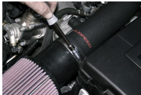
15. Install filter onto end of intake pipe and tighten clamp. Position NEUSPEED logo on end of filter horizontally for correct positioning.
