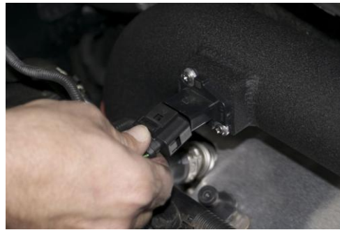
13. Attach MAF electrical connector.
