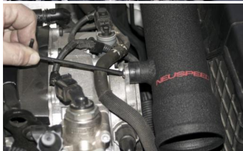
13. Attach MAF electrical connector.
