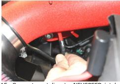
15. Connect vent line to *NEUSPEED* intake pipe.
