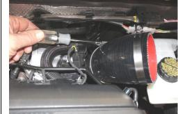
Install reduced end of 45° silicone hose 8. with #44 SS hose clamp onto turbo inlet, position hose so that opening is pointing directly toward left side of vehicle, then tighten clamp.
