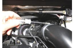
Disconnect air intake hose at turbo inlet using 7mm nut driver.
