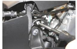
Remove T30 Torx screw from metal 9. support bracket on side of engine just below engine cover.
