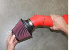
11. First loosely install NEUSPEED air filter onto intake pipe.
