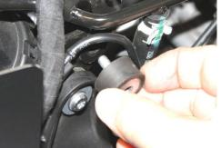
10. Install and hand tighten rubber isolator into threaded hole.
