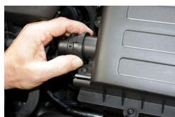
AIR PUMP ONLY: Squeeze collar to unlock and disconnect air pump hose from air filter box lid.
