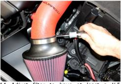
14. Adjust filter to have at least a  $\frac{1}{2}''$  clearance above heat shield, and then tighten with 8mm nut driver.
