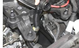
6. AIR PUMP ONLY: Pivot air pump hose to sit between the two front air box mounts.
