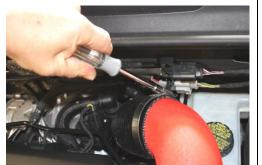
13. Tighten #48 SS hose clamp at intake pipe using 8mm nut driver.
