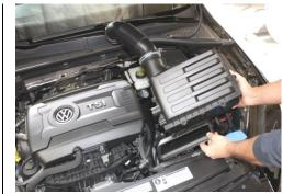
4. Lift out factory air filter box from its (3) rubber grommet mounts.
