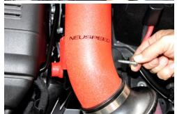
12. With #48 SS hose clamp loosely on silicone hose install *NEUSPEED* intake pipe, push on all the way until silicone hose meets bend in pipe. Then using supplied M6x30mm bolt attach pipe to rubber isolator and tighten.
