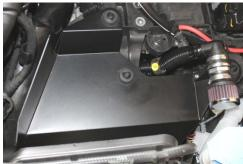
7. Install NEUSPEED heat shield onto original air box mounts. NOTE: Use WD-40 or equivalent on rubber grommets to ease install. Vehicles with air pump connect hose to billet fitting.
